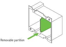
Install gang boxes that include vertical partitions (available at local electrical distributor) unless Class 2 circuit conductors are installed.
